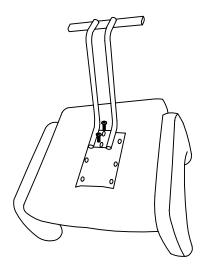
5. Insert the top of the hydraulic pump into the central hole underneath the seat. Place the chair on a level surface and press down on both armrests until the seat is secure.
