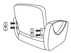
4. Remove the two preinstalled M5×20 bolts from the footrest. Fit the footrest onto the bottom of the seat and replace the two bolts to secure it. Tighten the bolts with the M5 hex wrench.
