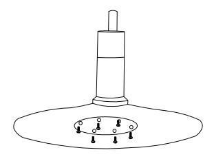
2. Loosen the preinstalled set screws on the pump using the M4 hex wrench. Fit the pedal onto the pump and secure it by retightening the screws.
