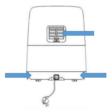
The diagram left shows the rear of the air fryer and the location of the air vent outlets (arrowed).
