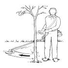
To free a blade that is bound in the cut, stop the unit, and support the trimmer or brushcutter to keep stress off the blade. Push the tree away from the entry point of the cut to open the cut, and pull the blade directly away from the cut in a straight-line motion. Use caution when releasing the tree to avoid being struck by spring-back or falling.
