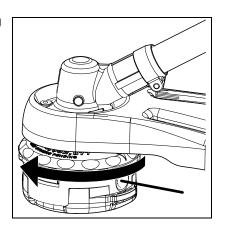
When the wear indicators located at the bottom of the Speed-Feed® head are worn smooth, or if holes appear, replacement of the cover or the entire Speed-Feed® head reauired.
