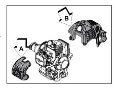
DO NOT use a metal scraper to remove dirt from the cylinder fins.
