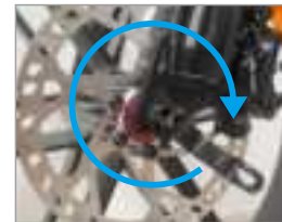
4. Rotate the quick release handle and lock it tightly
