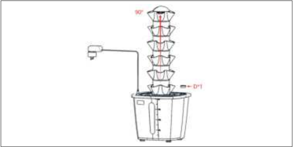
Figure 8: The water storage bucket is poured into the 20 liter nutrition solution with a folding funnel, the water inlet nozzle is covered, the intelligent switch is inserted into the power supply, and the balance of the foot is adjusted to 90° so that each layer of the water tower has the nutrient solution flowing through, then it can be used normally.
