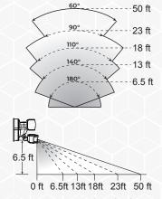
Recommended wall mounting height is at 6.5 ft. Environmental testing temperature: 25°C
