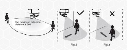
5. The sensor is very sensitive to lateral motion, with a maximum detection distance of 50 ft. (Fig. 2)
