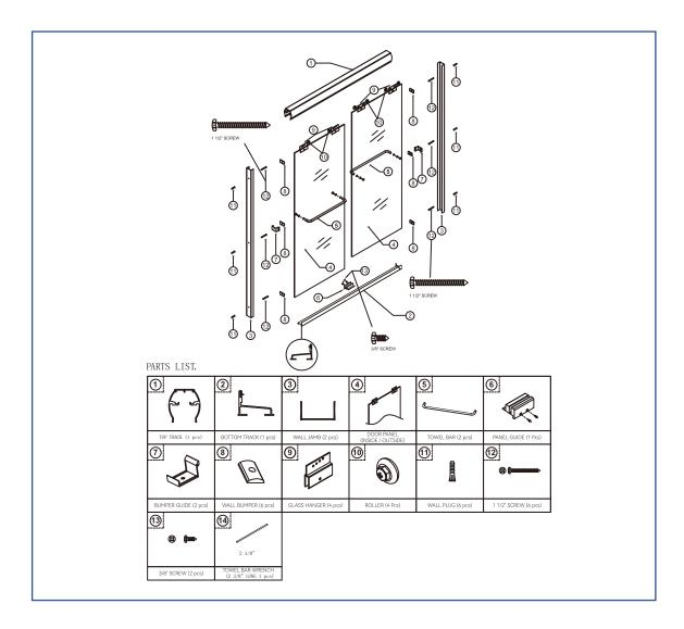
MATERIAL: All Hardware – 304 Stainless Steel and Aluminum Material
