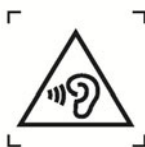
Figure 1 – Warning label (IEC 60417-6044)
