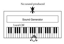
→ When connecting a unit in the Roland MT series, you don't need to switch off Local Control. MT units transmit Local Off messages when their power is switched on. If you first switch on the KR-7/5, then the MT-series device, Local Control is automatically switched off on the KR-7/5.
