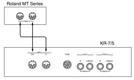
\* When the KR-7/5 is connected to a MIDI sequencer, set it to Local OFF. Refer to "Disconnecting the Keyboard from the Internal Sound Generator (Local On/Off)" (p. 160).
