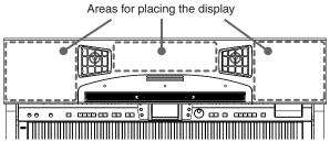
• If you are placing the display on top of the KR, we recommend using a liquid crystal display (LCD). If using a cathode ray tube (CRT) display, take extra care to ensure that the display rests stably on the instrument.
