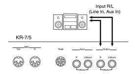
1. Turn the volume all the way down on the KR-7/5 and on the device you're about to connect.
