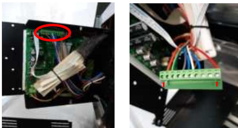
**Step 7:** Connect the flowmeters' cable to the screw terminal as follows: green wire (group 1) to position 4, white wire (ground) to position 5, and purple wire (group 2) to position 6. Short-circuit the three remaining wires (white, grey, and yellow) and use the provided heat-shrink to protect and isolate the connection. Use a cable-tie to secure and stress relief the cable.
