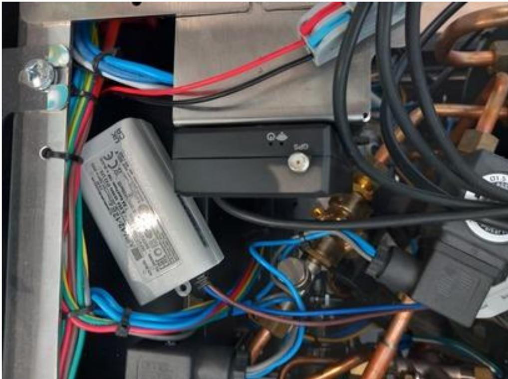
**Step 11:** Mount the magnetic GPS antenna at the top-right side of the coffee machine as shown below.
