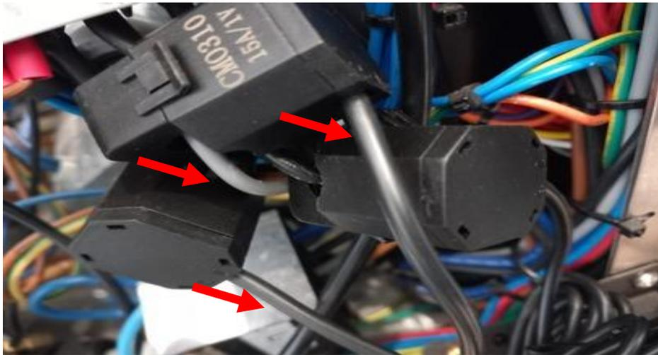
**Step 9:** Connect the blue (pump) CT to the power (live) cable of the pump, located at the left side of the machine, as shown below.
