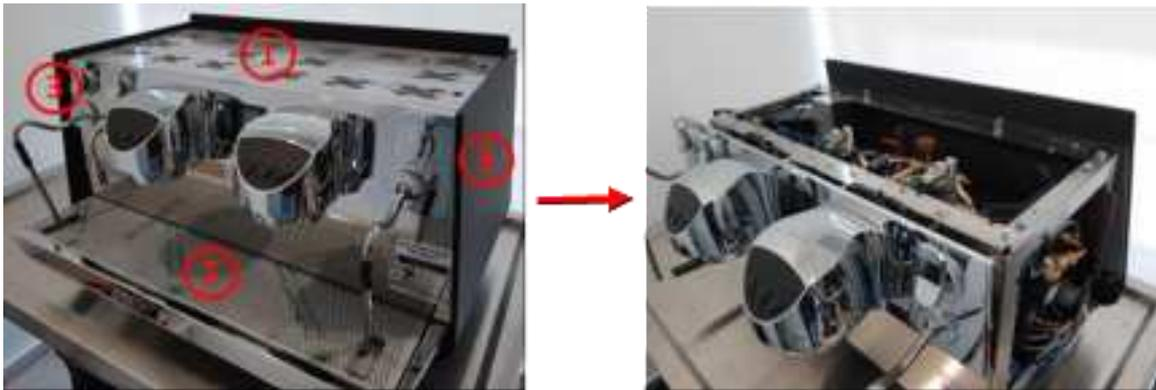
**Step 2:** At the left side of the machine, remove the screw highlighted in the picture below (left) to release the electronics' box and then remove the two screws on the top-left of the machine to release the power relay.
