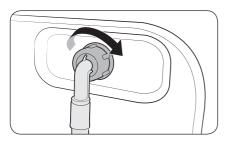
2. Connect the other end of the water hose to the inlet valve on the back of the washing machine, and then turn it to the right to tighten.
