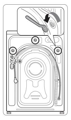
1. Locate the shipping bolts (marked with circle in the figure) on the rear side of the washing machine.
