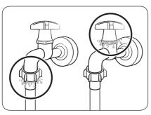
3. Slowly open the water tap and check if there are any leaks around the connection areas. If there are water leaks, repeat step 1 and 2.
