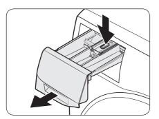
1. While holding down the **release lever** inside the drawer, slide open the drawer.
