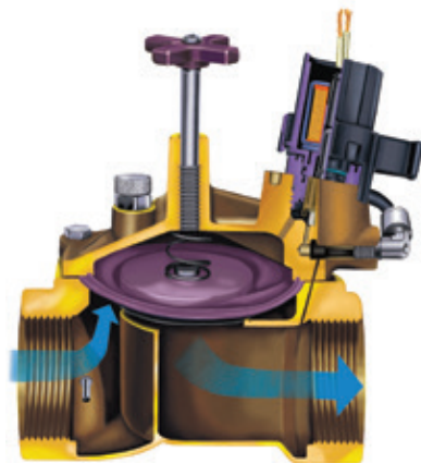
EFB-CP Cutaway
