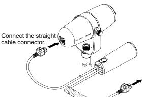
Connect to the transceiver with the 8-pin modular microphone connector.
