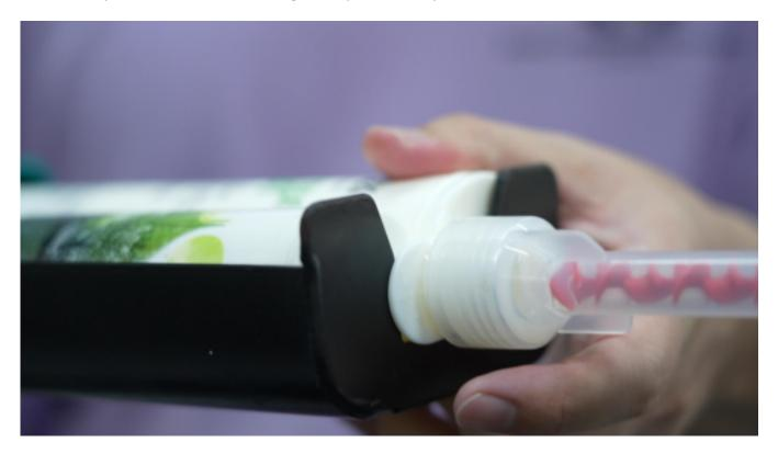
Lock the cartridge neck in position to fix well.
