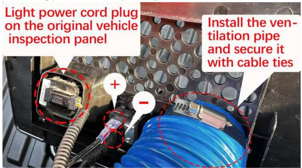
10. Replace the stock access panel with a venting and cooling panel with the power cord connected to it, and install it in place
