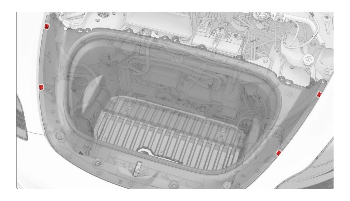
7. Route the 6 meter power cord from the rear tailgate cigarette lighter (do not connect the power first) through the hole shown in the picture to the front trunk and secure the power cord.
