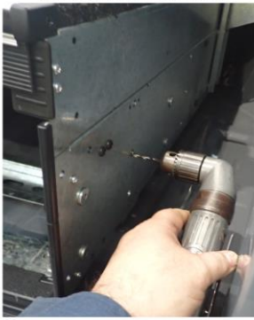
Pilot drilling of marked hole locations
