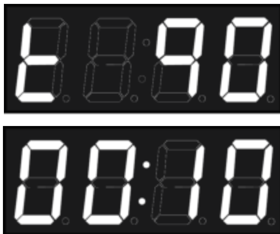
Figure 20. Example. Cooking at 90°C for 10 minutes
