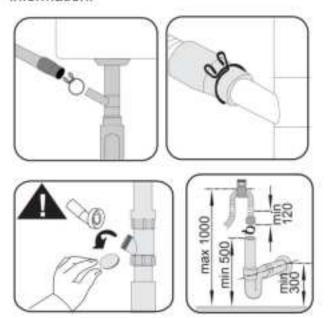
Drain pipe must be connected to the sewage system and it should not be connected to any surface water.
