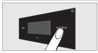
■ To switch on: press the ① button. The ⊞□⊜, ⇔ and Start/Stop sensor controls and the sensor controls in the display react to finger tip contact.
