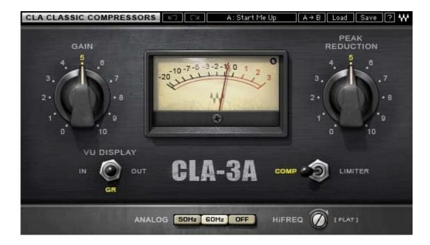
The CLA-3A offers 2 main controls for compression, as well as additional controls for fine-tuning.
