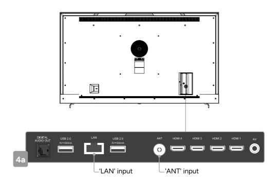
Following these options, the **Auto Tuning** screen will appear. Ensure you have an antenna cable connected to the 'ANT' input port at the back of the TV **(4a)**.
