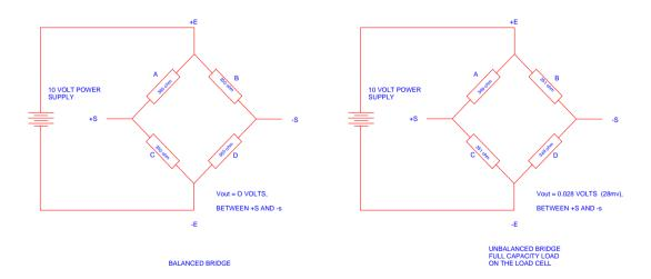
This will cause the bridge to become unbalanced. When the bridge has a voltage across it from +E to -E then the signal output at +S and -S will show a voltage of zero volts with no load and a small voltage proportional to the load as the load is increased. Typical load cells show 20-30mv of signal if the excitation voltage is 10volts and the load cell is fully loaded.
