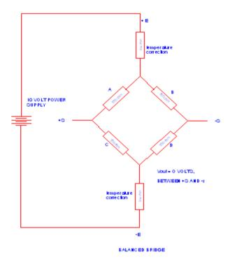
A method to check the basic function and integrity of a load cell can be done using an ohmmeter and voltmeter with up to a 10volt power supply.
