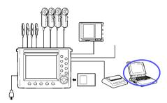
The 3169-20/21 includes an RS-232C interface as standard equipment. Using the RS-232C interface, settings of the 3169-20/21 can be made and measurement data can be acquired on a PC. This chapter explains how to connect the 3169-20/21 to a PC. For details including communications commands, see the RS-232C instruction manual (CD-R version).
