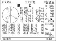
Wiring check screen (Power factor: 0.87)
