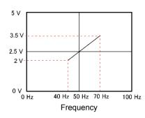
The D/A terminal outputs approximately 6.6V at the frequency other than between 40 and 70 Hz.
