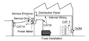
Using a measurement product in an environment designated with a higher-numbered category than that for which the product is rated could result in a severe accident, and must be carefully avoided. Use of a measurement instrument that is not CAT-rated in CAT II to CAT IV measurement applications could result in a severe accident, and must be carefully avoided.
