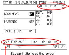
Displays the number of output data items. Make sure the number of output data items does not exceed 256 when reading stored data into a generally available spreadsheet.
