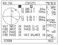
Wiring check screen (Power factor: 1) 4.2.5 Checking the Wiring (page 52)
