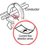
The arrows on the clamp indicating the direction of current flow should point toward the load side.
