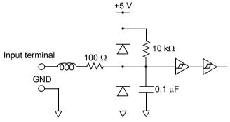
An 0/5-V logic signal or short/open contact signal is used for control.
