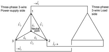
The figure above shows an artificial circuit of a three-phase 3-wire line. In the figure,  $\dot{U}_1$ ,  $\dot{U}_2$ , and  $\dot{U}_3$  represent the vectors of line to line voltage;  $\dot{I}_1$ ,  $\dot{I}_2$ , and  $\dot{I}_3$  represent the line (phase) current vectors;  $\dot{u}_1$ ,  $\dot{u}_2$ , and  $\dot{u}_3$  represent the phase to neutral voltage vectors. Normally, three-phase power P is obtained as the sum of the power of the phases.
