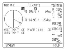
Wiring check screen (Power factor: 0.87) 4.2.5 Checking the Wiring (page 52)
