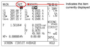
Changes the circuit to display (when multiple circuits are measured).
