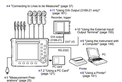
\*: The RS-232C is connected to a printer or PC.
