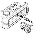
To connect the 3169-20/21 to a PC, you need the optional 9612 RS-232C cable. The 9612 RS-232C cable is a cross cable.
