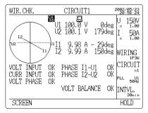
Wiring check screen (Power factor: 0.87)
