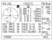
Wiring check screen (Power factor: 0.87)
