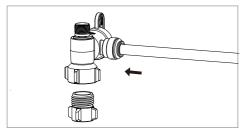
(C) Install the Angle Stop Valve on the cold water valve and tighten it with an adjustable wrench. Please don't miss the gasket inside the angle stop adapter during installation.
