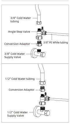
(D) Switch off the angle stop adapter. Turn on the cold water supply valve. Wipe the connections with a tissue to check for leakage. If the tissue stays dry, the angle stop valve is installed correctly.
