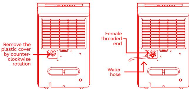
**Note:** Do not use continuous draining when the outdoor temperature is equal to or less than 32°F (0°C), otherwise the water will freeze, causing the water hose to block up and the dehumidifier may be damaged.
