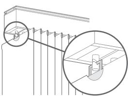
Hook the control wand onto the eyelet at the end of the hooks. Note that the control wand will be located according to which side you chose to 'stack' the blind on. Most blinds will have a single wand, but wider blinds provided with two headrails will comprised of one left-stack blind and one right-stack blind, so there will be two wands in the centre.
