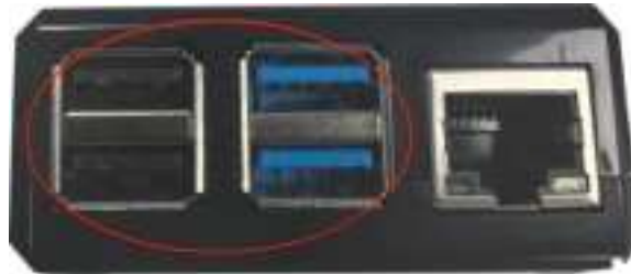
Figure 3 Data ports on Element-D
