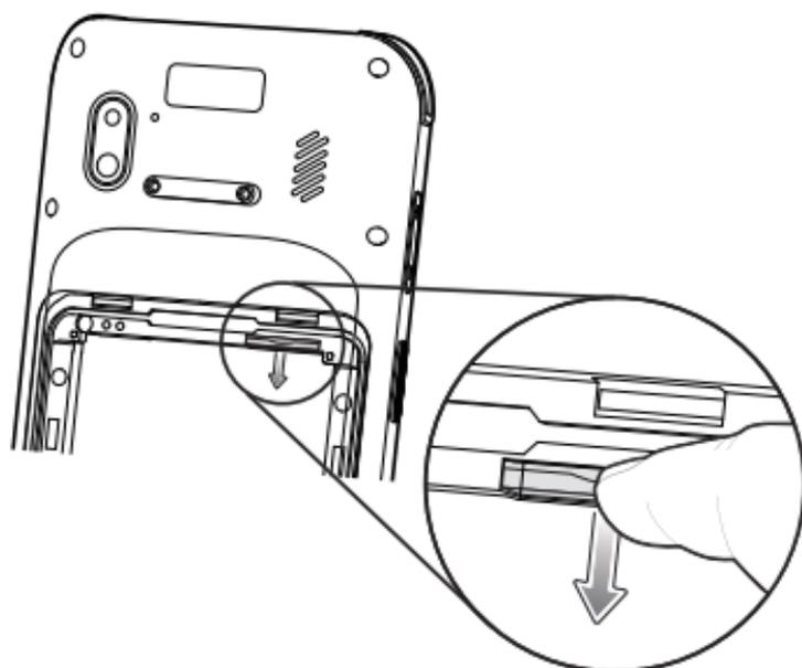
6. Remove the SD/SIM card drawer from the device.
