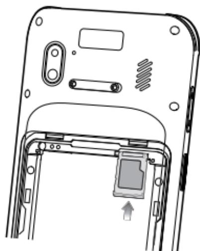
10. Press the SD/SIM card drawer into the device to ensure it is in securely.
