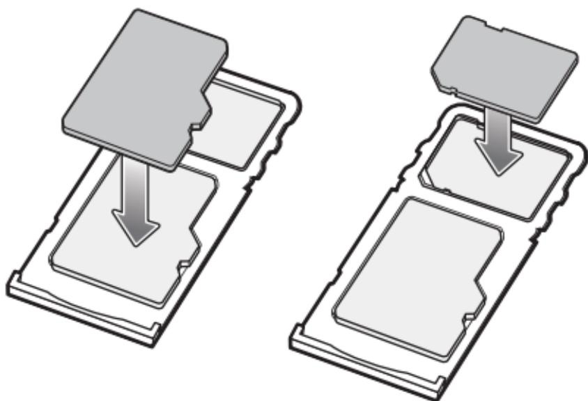
8. If you are using two SIM cards, insert the second SIM card into the microSD card slot.
