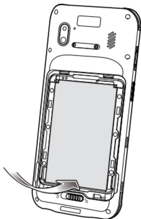
14. Insert and align the cover into the bottom latches
