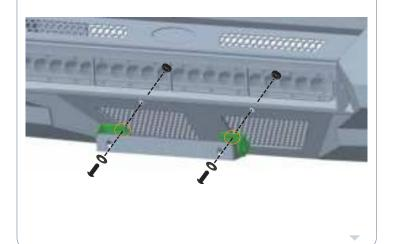
Install the mounting bracket onto the bumper. Repeat this step for the other side. Tighten the hardware.
