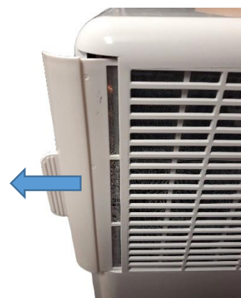
Above: The Air Filter located on the top left hand side of the unit (shown partially removed). To remove, slide the filter out in the direction of the arrow.
