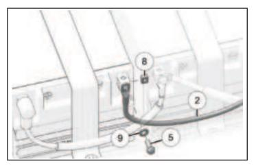
8. Install secondary and NEGATIVE (–) battery cables to primary battery with one battery nut, one washer, and one battery terminal fastener.
