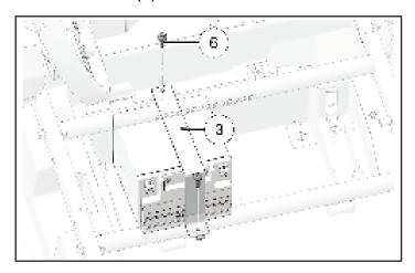
4. Replace primary battery and secure with battery bracket and two fasteners.
