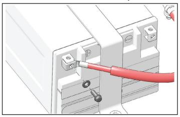
3. Remove and retain two battery bracket fasteners to remove battery bracket.
