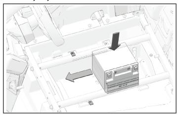
3. Secure battery to battery tray with bracket (3) and two fasteners (6).
