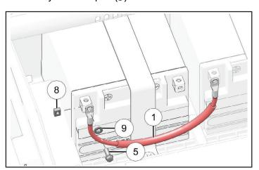
6. Install secondary and primary POSITIVE (+) battery cables to primary battery with one battery nut, one washer, and one battery terminal fastener.
