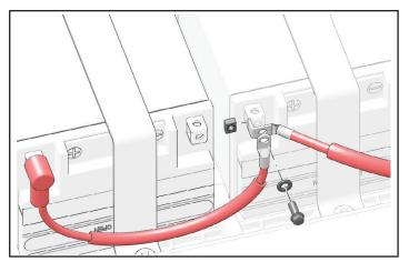
7. Install NEGATIVE (–) battery cable (2) to battery with one battery nut(8), one washer(9), and one battery terminal fastener
