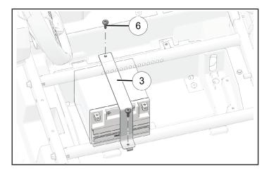
4. Replace primary battery and secure with battery bracket and two fasteners.
