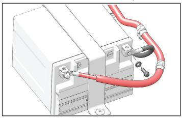
2. Remove and retain battery terminal fastener and washer to remove POSITIVE battery cable.
