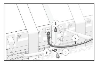
8. Install secondary and NEGATIVE (–) battery cables to primary battery with one battery nut, one washer, and one battery terminal fastener.
