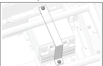
4. Maneuver primary battery out of battery compartment.
