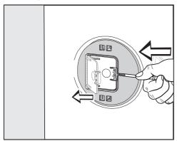
■ Push against the catch with a pointed object, e.g. a narrow screwdriver.
