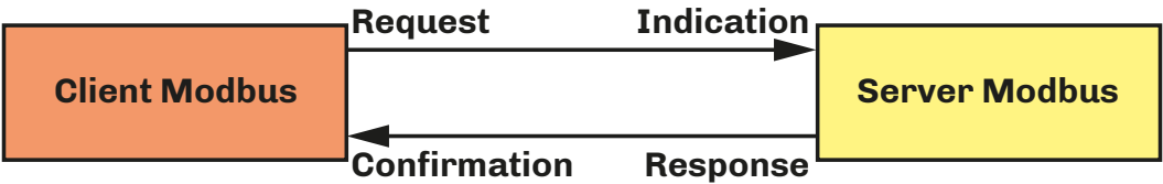
Fig. 35. Diagram showing message exchange in a Modbus TCP communication
