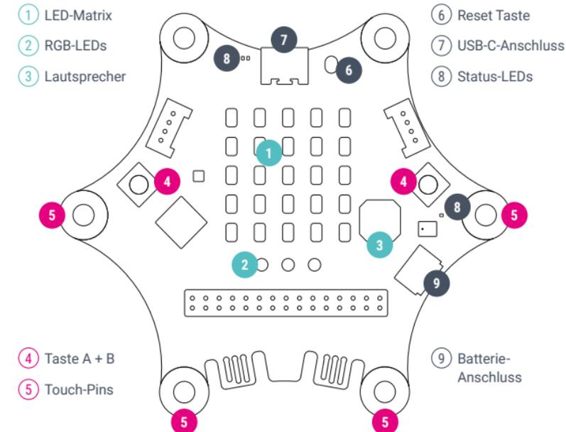
EN: Display, RGB-LEDs, Speaker, Buttons, Touch-Pins, Reset, USB, Battery, Status-LEDs
