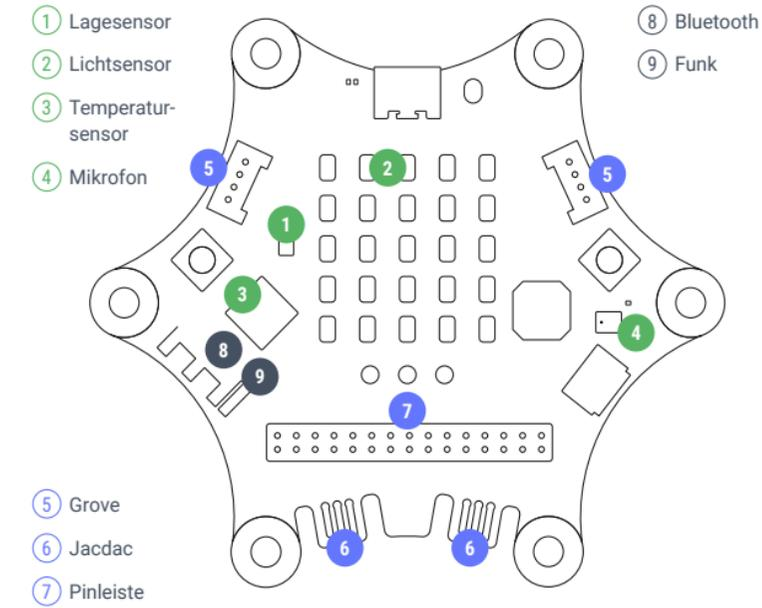
EN: Motion-, Light-, Temperatur Sensor, Mikrofon, Grove, Jacdac, Pins, Bluetooth, Radio
