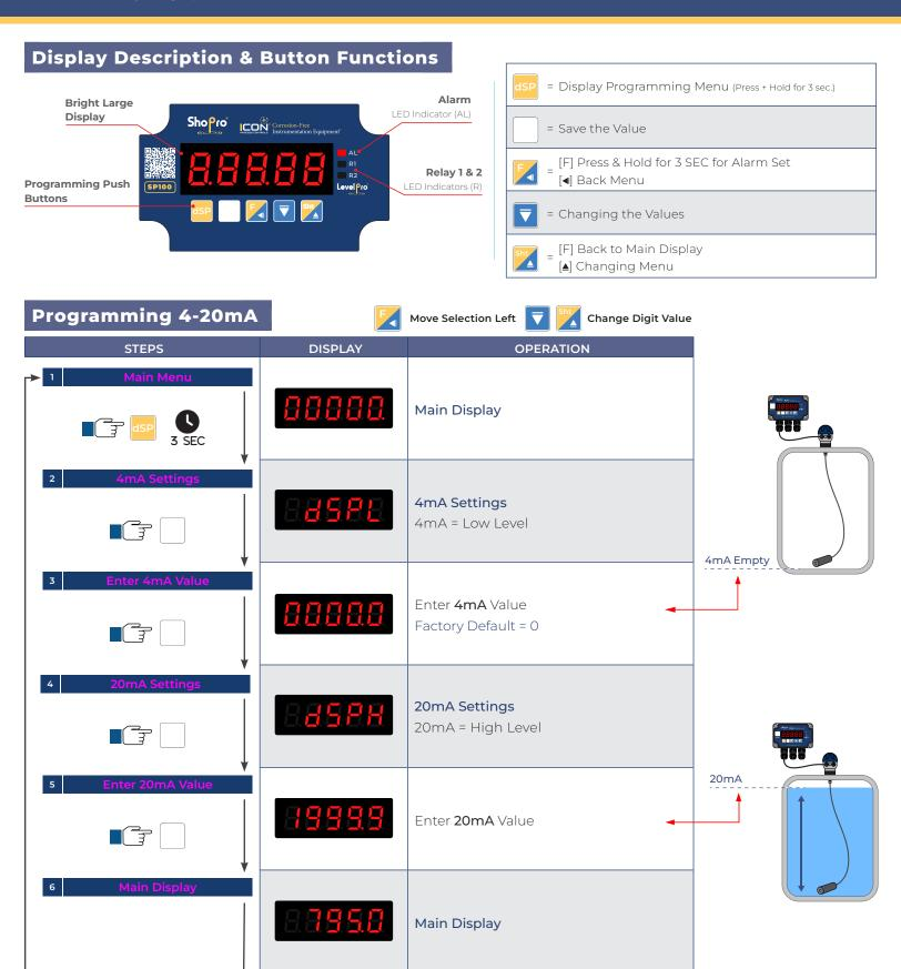
dSPL = Low Level Value | Empty or Lowest Liquid Level | Factory Default = 0. dSPH = High Level Value | Enter Maximum Level.
