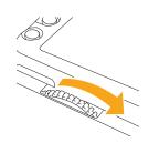
5. Rotate the thumbwheel in the direction of the arrow until the grip is secured to the camera.
