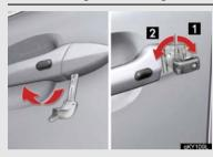
To unlock or lock the vehicle, use the mechanical key to remove the lock cover on the driver's door handle. The mechanical key is stored inside the electronic key.
