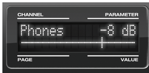
Figure 6-4: The LCD provides feedback as you adjust volume.
