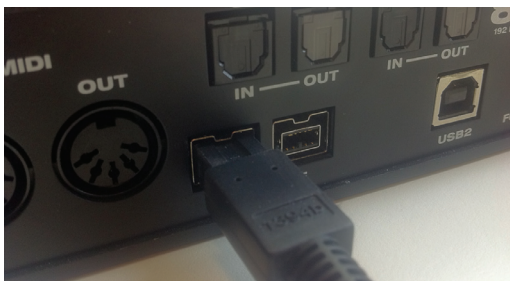
Figure 4-1: Connecting the 828mk3 to the computer via FireWire.
