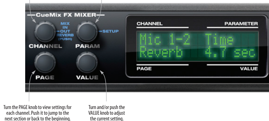
Figure 6-3: The 828mk3 front panel controls.
