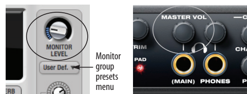
Figure 9-24: Monitor group volume control from CueMix FX and the front panel MASTER VOL knob.
