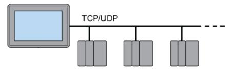
Connection in a network is made according to Ethernet standards.
