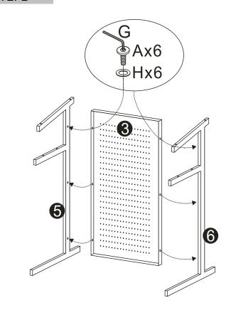
Connect left leg ⑤ and right leg ⑥ to back panel ③ with 6 pcs screws A and tighten them with Allen wrench G
