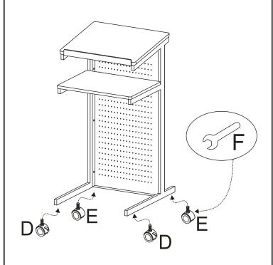
Install 2 pcs wheels with lock D at the front, install 2 pcs wheels E at the back, and tighten them with wrench F
