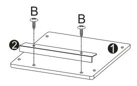
Fix the cross bar ② on the top board with 2 pcs screws B
