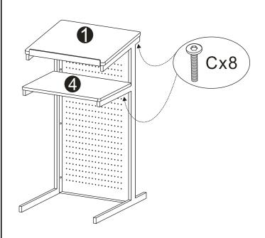
Fix the top board  $\ensuremath{\textcircled{1}}$  and shelf  $\ensuremath{\textcircled{4}}$  to legs with 8 pcs screws C
