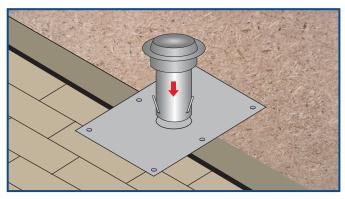
2. Align Cap Slots with Base Tabs, then Lower cap onto conical base.
