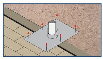
1. Shingle up to the exhaust pipe then slip on base flashing. Secure with 6 roofing nails.
