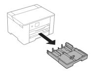
2 Slide the side edge guides all the way out and set the front edge guide to the paper size you are using.
