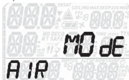
When selecting Nitrox, you can define the percentage of oxygen in the mixture (O<sub>2</sub>%) and the maximum value of oxygen partial pressure (ppO<sub>2</sub>max) for up to three breathing mixes. The maximum possible value for the ppO<sub>2</sub>max is 1.6bar. Most training agencies recommend not to exceed a value of 1.4bar.
