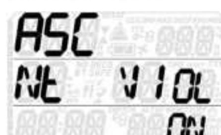
If the ascent rate exceeds 120% of the allowed value over a depth change of more than 20m/66ft, due to the potential of harmful bubble formation, Quad 2 locks the computer for 48 hours in order to prevent you from diving
