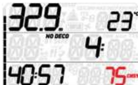
If the oxygen toxicity level reaches 75%, ascend to shallower depth to decrease oxygen loading and consider terminating the dive.
