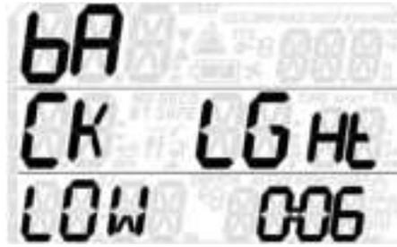
This menu allows you to set the duration of the backlight between 2 and 12 seconds. Default setting is 6 seconds.
