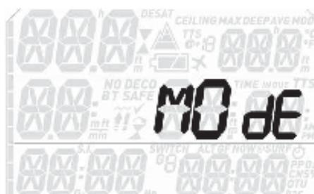
In this menu you define the type of gas you will be breathing during the dive (**AIR** as **SINGLE GAS**, **NITROX** as **SINGLE GAS**, **NITROX** as **MULTIGAS**, **TRIMIX** as **MULTIGAS**). You can also set Quad 2 to **BOTTOM TIMER**, in which case Quad 2 will show only time, depth and temperature: it will not carry out any decompression calculation and it will not show any warnings and alarms.
