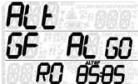
Quad 2 allows you to define an alternate set of gradient factors, to use when you need to cut your decompression short in case of an emergency. The set of alternate gradient factors cannot be more conservative (i.e. lower) than the main set of GF values. The default value is R0 (85/85).
