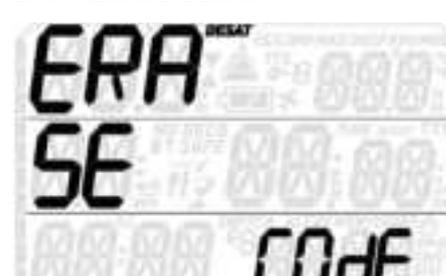
Quad 2 allows you to reset the desaturation in the computer. Any tissue saturation information from a recent dive will be reset to zero and the computer treats the next dive as a non-repetitive dive. This is useful when the computer is loaned to another diver who has not dived in the last 24 hours.
