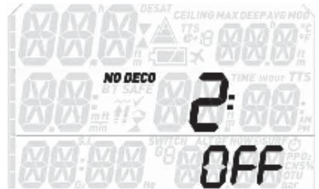
When this is set to **ON**, a warning will alert you when the NO STOP time reaches 2 minutes.
