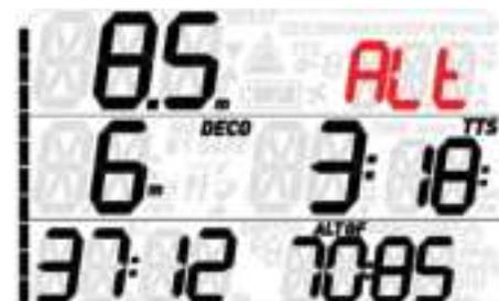
If the alternate gradient factors are not compatible with the current depth, Quad 2 considers this a dive violation and the deco violation symbol will appear, blinking, until you press any button to acknowledge having seen it.
