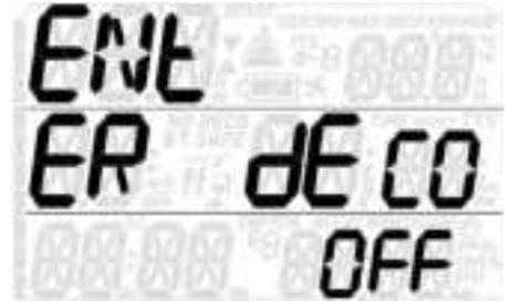
When this is set to **ON**, a warning will alert you when a mandatory decompression stop has been calculated by Quad 2.
