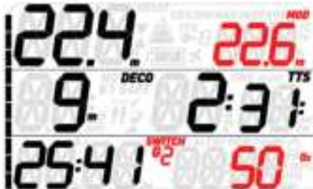
Use **BR-LP** to confirm the switch to G2: the set oxygen concentration will be displayed steadily in the lower right corner of the screen: if **PREDICTIVE** is set to **ON**, the decompression calculation will not change; if **PREDICTIVE** is set to **OFF**, within 20 seconds of having switched gas, the decompression calculation will be updated to reflect the change in gas.
