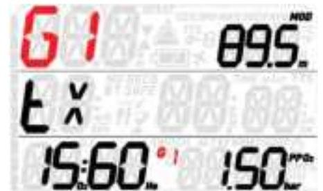
Quad 2 allows you to set up to 5 gases in which in addition to the oxygen percentage you can also set the helium percentage. Everything is the same as with multigas nitrox diving with the addition of OTUs (Oxygen Toxicity Units) in the sequence of data fields in the bottom right corner.
