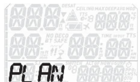
This function allows you to plan your next dive. In case you dived recently, with **TR-SP** you can enter an additional surface interval in 15-minute increments between now and when you intend to dive: the residual nitrogen load will be adapted accordingly. Quad 2 will consider all active gases and set gradient factors, displaying them at the bottom of the
