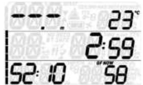
If you submerge again before the countdown is over, the dive time will resume from where it left off, including the time spent on the surface. If you do not submerge before the end of the countdown, Quad 2 considers the dive finished, records the data to the logbook and reverts to the so-called **POST DIVE** mode.
