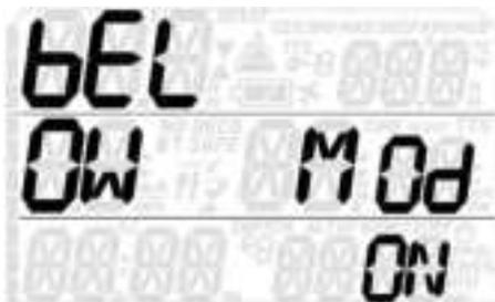
When set to **ON**, Quad 2 will allow a switch to a gas at a depth deeper than the MOD of the gas (resulting in an immediate MOD alarm).
