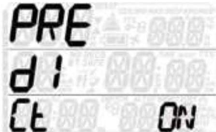
When set to **ON**, Quad 2 will consider all gases in the decompression calculation, with switches carried out at the MOD of each gas. When set to **OFF**, the decompression calculation will consider the currently breathed gas only. See Section 10 for more information about the **PREDICTIVE** feature.
