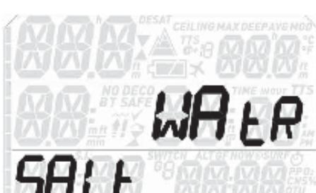
You can set the computer to fresh water, salt water or **EN13319** calibration, depending on where you intend to dive. Setting the wrong water type entails an error in depth measurement of maximum 3% (i.e. at a depth of 30m/100ft, a computer set to salt
