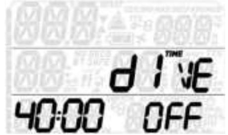
Quad 2 allows you to set a time alarm, triggering also a warning at half of the set time limit. The default value is **OFF**. Using the button, you can set the value between 20 and 90 minutes in 2-minute increments. Upon reaching half of the set limit, the dive time will blink until you hit any button to acknowledge it. Upon reaching the set time limit, the dive time again blinks until you hit any button to acknowledge it.
