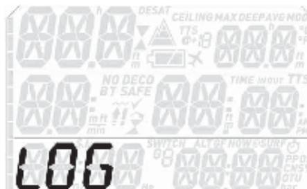
Quad 2 can record the profiles of over 100 hours of diving, at a sampling rate of 5 seconds. The information can be transferred to a Smartphone (Mares or MySSI app, via bluetooth). In addition, Quad 2 can show most of the information directly on the display. Upon entering the logbook you will see **StAt**. Entering this menu will show the
