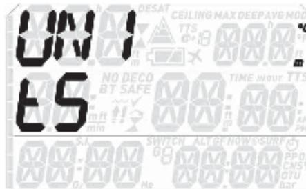
You can choose between metric (depth in meters, temperature in °C), and imperial (depth in feet, temperature in °F).
