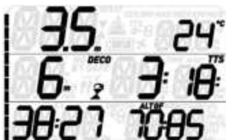
In this case, if the diver attempts a repetitive dive after surfacing, Quad 2 will function only as a depth gauge and timer (bottom timer mode) and it will display the missed deco stop violation symbol (⚠).
