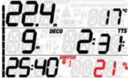
Use **BR-SP** while this indication is blinking to initiate the gas switch: the oxygen percentage of G2 starts to blink in lieu of that of G1, and in the top right corner the MOD of G2 is displayed, also blinking.
