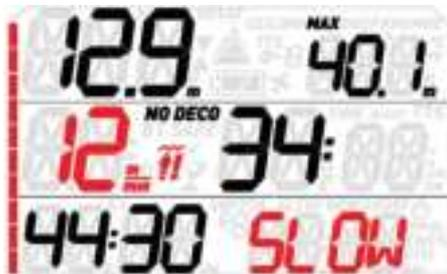
This persists until the ascent rate is reduced to below the pertinent limit. The limits are dependent on the current depth as follow:
