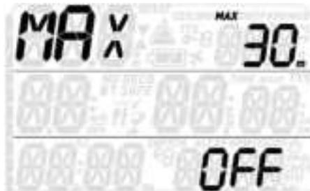
Quad 2 allows you to set an alarm at a depth independent of the MOD. The default value is **OFF**. Using **TR-SP** or **BR-SP** you can set it between 10m / 30ft and up to just shy of the MOD, in 1m / 5ft increments. Upon reaching the defined depth an alarm similar in behaviour to the **MOD** alarm (section 7.3.2) is triggered. Press any button to acknowledge having seen it.
