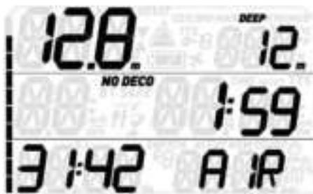
DECO stops are generated progressively as you stay at depth beyond the no deco time. DECO stops are **MANDATORY**. As you approach the depth of a stop, the duration of the stop is gradually reduced. The duration itself is always shown in minutes, and is calculated as a function of the pressure gradient achieved at the stop depth itself. Hence the farther you are from the exact depth of the stop, the longer it will take for each minute to tick off.
