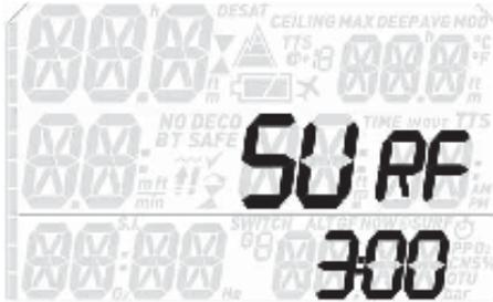
In this menu you can set the duration of the interval from the moment you reach the surface to when the dive computer closes the dive. During this interval you can submerge again and resume the dive. This menu allows you to change the default 3-minute interval to any value between 1 minute and 45 minutes.
