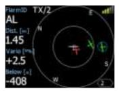
Middle buttons help with target selection by cycling through available targets. Lower button has ZOOM back or EDIT function with long press, where we can edit/view the currently selected target.
