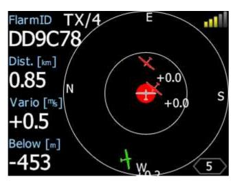
All targets are displayed as a glider symbols. User can change that symbol to another type. It's alsp possible to change object color, depending on relative altitude to us. All received targets (Flarm or PCAS) are marked with same type of symbol except undirected targets, for which we don't know from which direction they are comming from. Flarm targets can be separated only by their ID.
