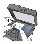
2 Align it flush against the original size indicator plates with the back left corner as the reference point.
