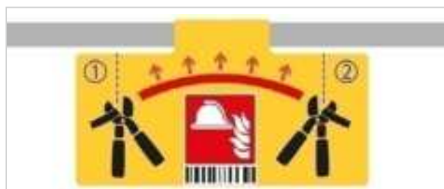
High-voltage rescue disconnect device information label (extract from rescue card)
