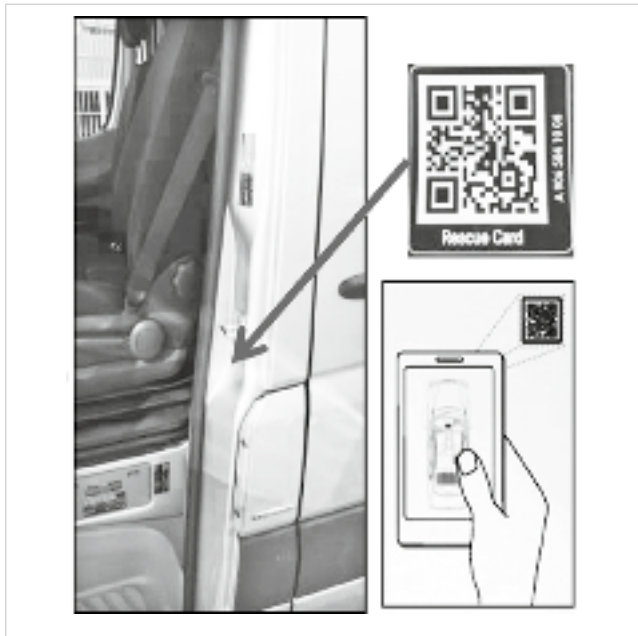
QR code rescue sticker on B-pillar on driver's side (example, schematic diagram)
