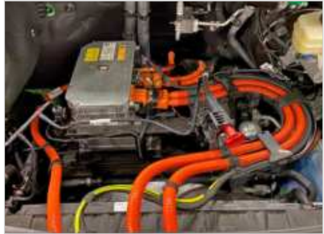
High-voltage lines in the engine compartment
