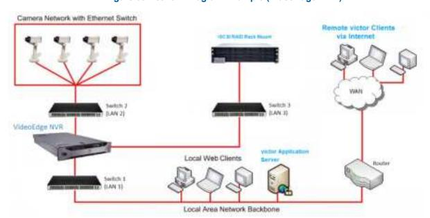
Figure 65 Network Diagram Example (VideoEdge NVR)
