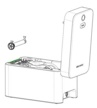
6.4.4 Use alcohol swabs or lint-free cloths to clean the print roller. Wipe from the middle area to the ends repeatedly until the print roller surface is completely clean. In case of excessive sticky substances or tightly stuck label paper, use new swabs to clean the residues.
