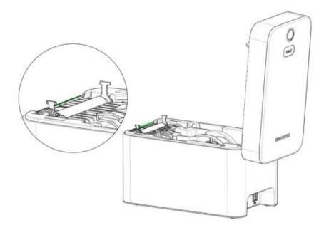
6.4.3 Pull the print roller upward and take it out of the bottom support of the printer.
