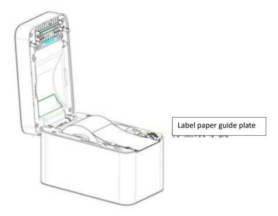
4.3.4 Close the paper compartment and press the lid gently until you hear a "click" sound. The lid is now locked, and the printer will retract the label paper automatically, indicating that the label paper has been loaded successfully.
